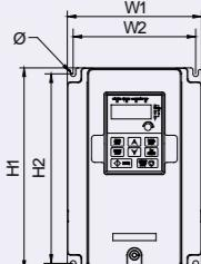
Wall mounting of 3PH 380V 4~37kW and 3PH 220V 1.5~7.5 kW inverters
