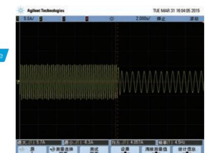
Current waveforms when sudden unloading in vector control mode with 0.5Hz and full load
