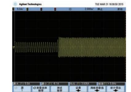
Current waveforms when sudden loading in V/F control mode with 2Hz and full load
